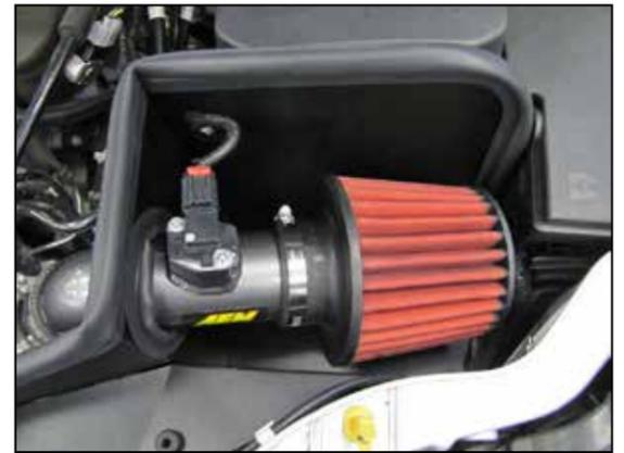
20. Route the MAF sensor wire harness through the heat shield cut out, then reconnect MAF sensor.
