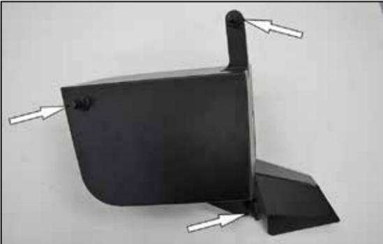
13. Install factory push in mount and the 2 AEM® air box mount to heat shield.
